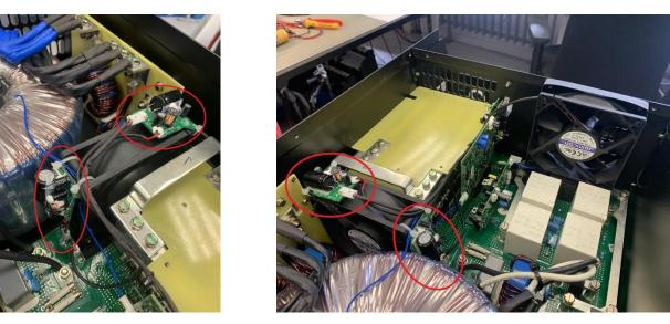
7. Check carefully that the converter PCBA(s) are installed correctly. Reconnect the AC and DC cables, replace covers and switch the unit ON to test. Put the inverter or charger under maximum load to test the fan(s).
